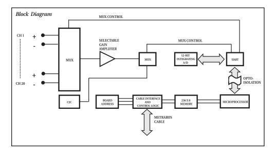
20-Channel Thermocouple Interface Board For the METRABUS
