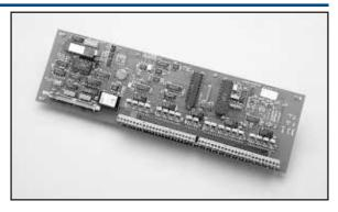
The MTHERM-20 is fully isolated to 500 VDC with greater than 72 dB Common Mode Rejection (35 dB NMR). Measurement resolution is 0.1 to 0.8°C (range dependent) with a measurement accuracy of 0.5°C. Signal input filtering can be implemented using a four sample-time constant (switch-selectable). Required power is +5 VDC @ 500 mA (typ) via the METRABUS cable or via an external power supply. Removable screw terminals will accept 14 AWG or smaller thermocouple wire.
